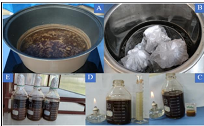
Figure 1. Pretreatment and hydrolysis process: (A) Boiling, (B) Using autoclave, (C) Adding cellulase enzyme, (D) Adding algal enzyme, (E) Using a solar dryer
